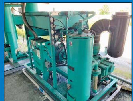
100-HP Sullivan Model 1000D Skid Mounted Rotary Screw Air Compressor
